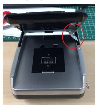
Sometimes it happens that, when closing the device, the cable gets 'in the way':
