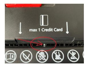
Check if you can move that clip (with a knife for example) If it is jammed, then the shredder will not start, then you must clear the jam
