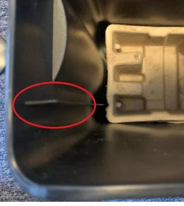
The plastic line in the waste bin should be undamaged
